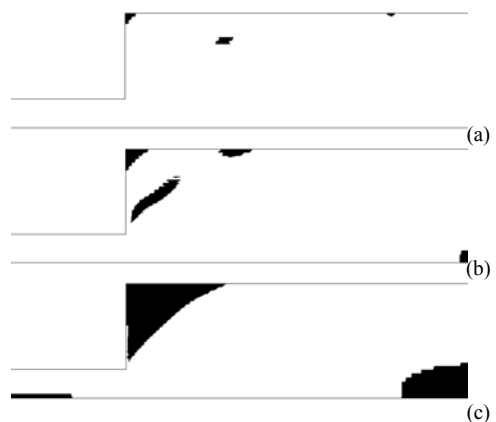
Figure 4: Structure of the unyielded zone, Re=50 . (a) Ca=0.1 , (b) Ca=0.8 , (c) Ca=1.5
